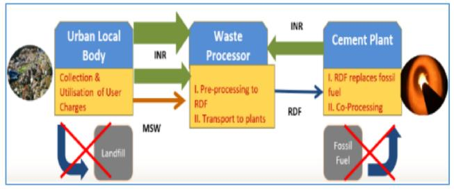
Figure 13. Flowchart of MSW to RDF plant to RDF co-processing in cement kilns
