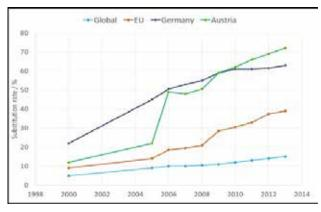
Figure 5: Thermal substitution by alternative fuels in the cement industry<sup>6</sup>
