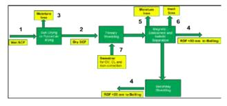
Figure 15 Process block diagram for manufacturing RDF from SCF
