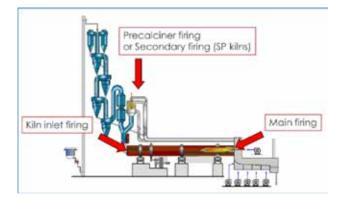
Figure 16: Options for fuel feed points at cement kiln<sup>55</sup>
